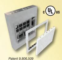
The PWB-450 and PWB-FR-450 (Fire Rated model) mount in a typical 4" deep wall between the studs in a standard 16" stud bay. They provide connectivity, internal device mounting and power in a secure and invisible manner. The wall box has four pre-wired AC outlets, four accessory plate mounting brackets and included IPS and Decora style accessory mounting plates. (Also see back page for other options for manufacturer specific product mounting).
