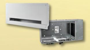
The **PWB-250** is approx.14.25"x7"x4" and has three single gang knockouts and one IPS knockout to mount up to six single IPS plates. A removable pass thru enclosure provides an additional single gang knockout to be used to isolate cables that may need to pass through the backbone.
