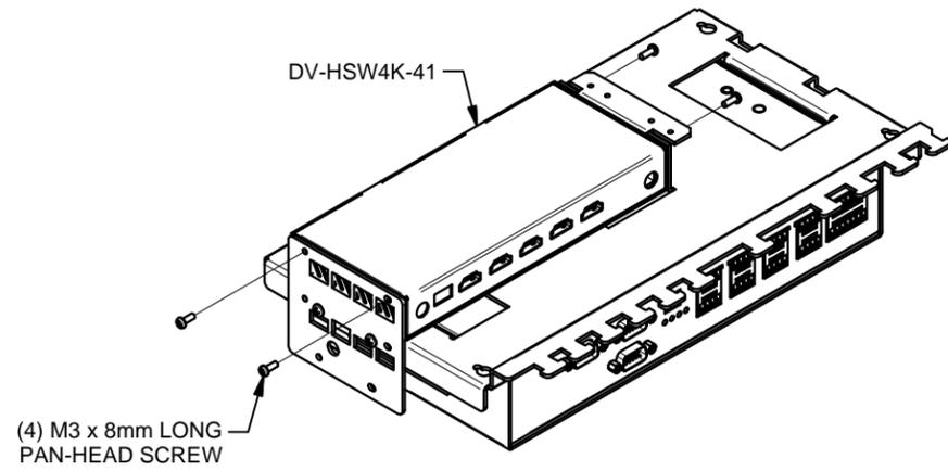
4B. INSTALLING TWO DV-HSW4K-41 UNITS:
