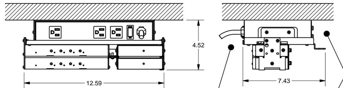
BE SURE TO PLAN FOR WIRING / CABLE ROOM IN FRONT & BACK OF ASSEMBLY
