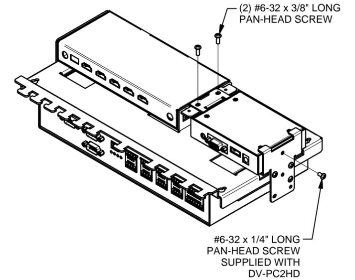
5B. INSTALLING TWO DV-PC2HD UNITS:
