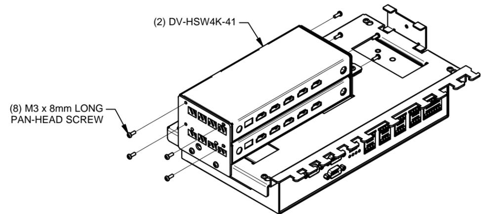
5A. INSTALLING ONE DV-PC2HD UNIT:
