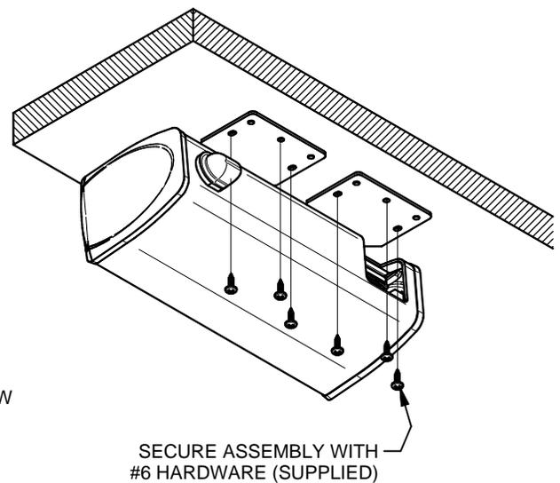
3. IF APPLICABLE, INSTALL KEYSTONE CONNECTORS (SOLD SEPARATELY) INTO INSERTS (SINGLE OR DUAL), MAKE WIRING CONNECTIONS AS REQUIRED, AND INSTALL INSERTS INTO ASSEMBLY. IF KEYSTONE CONNECTORS ARE TO BE INSTALLED AT A LATER DATE INSTALL BLANK INSERTS. FRONT FACE MUST BE CLOSED WITH KEYSTONE OR BLANK INSERTS.
