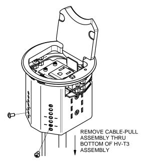
3. REASSEMBLE CABLE-PULL ASSEMBLY WITH SUPPLIED HD15 CABLE, 3.5mm STEREO CABLE, VGA/AUDIO CABLE TRAP, SPACERS AND #6-32 x 3/8 LONG FLAT HEAD SCREWS.
