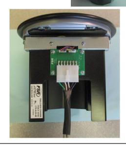
WIRING CABLE WITH "CONTACT IN" LABEL
