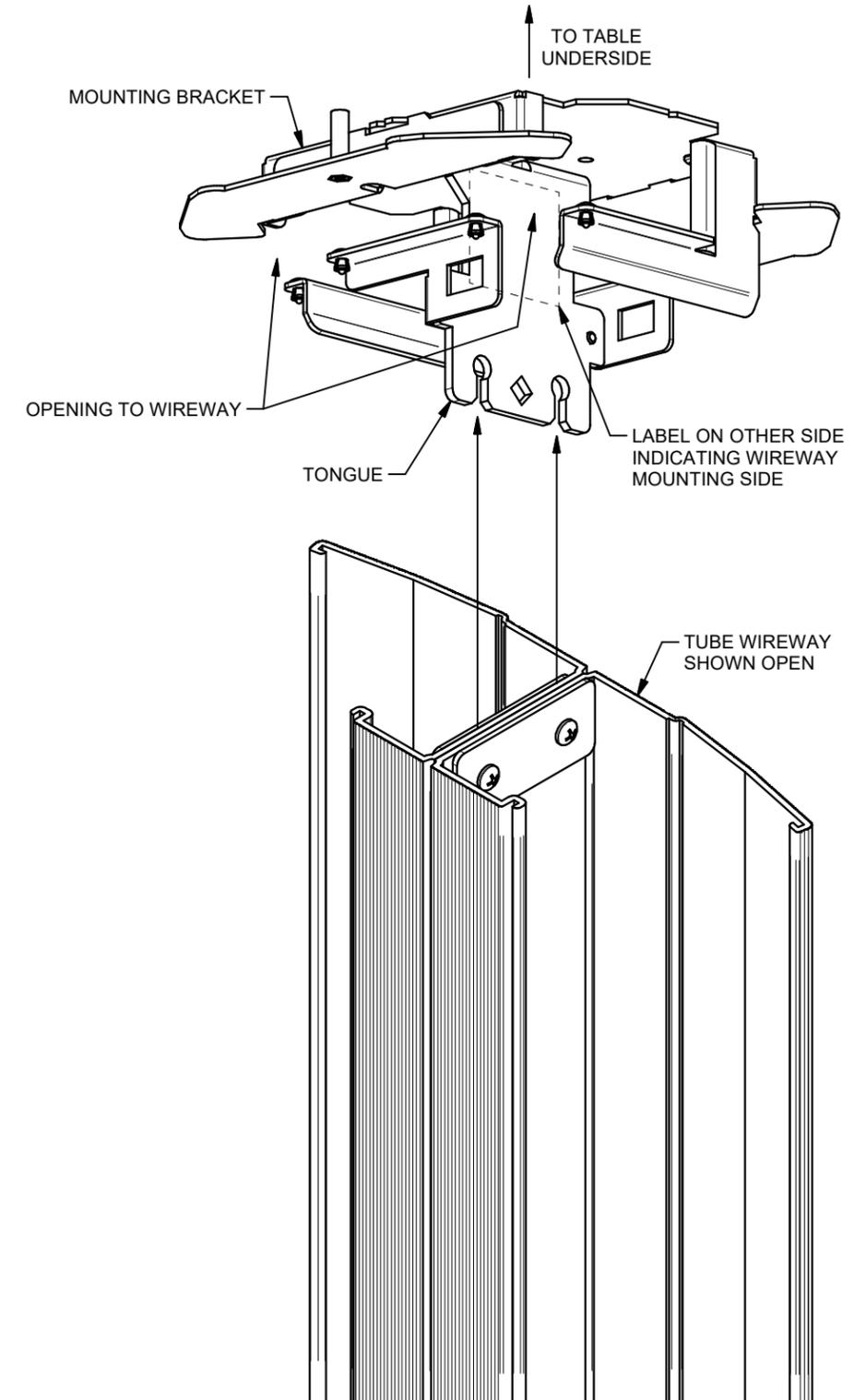
2. INSTALL MOUNTING BRACKET TO UNDERSIDE OF TABLE AS SHOWN.
