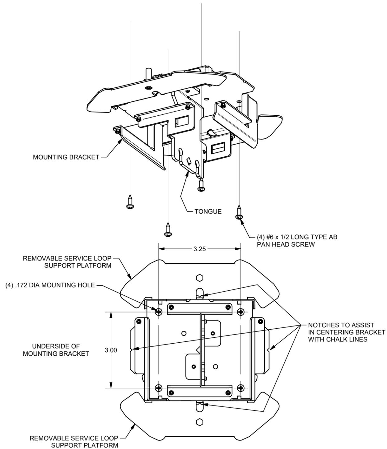
3. OPEN TUBE WIREWAY AND INSTALL MOUNTING PLATES AS SHOWN. THREAD THE SCREWS IN ONLY 1/8" SO THAT THE WIREWAY CAN BE INSTALLED ONTO TONGUE.
