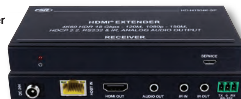
HD-H1504K-SP 18Gbps HDMI extender set tha allows HDMI, RS-232, and bi-directional IR signals to be extended to a distance up to 492ft / 150 meters between the transmitter and receiver via a single CAT cable
