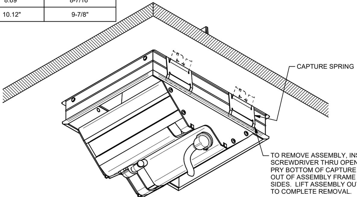
2. IF APPLICABLE, INSTALL KEYSTONE CONNECTORS (SOLD SEPARATELY) INTO INSERTS (SINGLE OR DUAL), MAKE WIRING CONNECTIONS AS REQUIRED, AND INSTALL INSERTS INTO ASSEMBLY. IF KEYSTONE CONNECTORS ARE TO BE INSTALLED AT A LATER DATE INSTALL BLANK INSERTS. FRONT FACE MUST BE CLOSED WITH KEYSTONE OR BLANK INSERTS.
