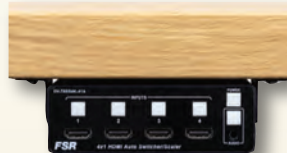
Quad Digital retractor kit gives you button control on the table box with the 1U height presentation switcher mounted
