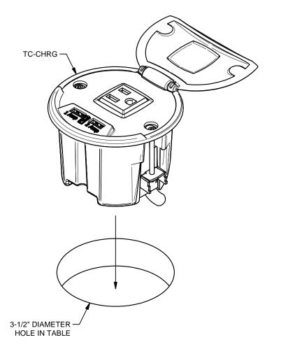
SECURE TC-CHRG ASSEMBLY TO TABLE BY TIGHTENING MOUNTING SCREWS. ALTERNATELY TIGHTEN LEFT AND RIGHT SCREWS TO MAINTAIN CENTERING OF ASSEMBLY IN TABLE.
